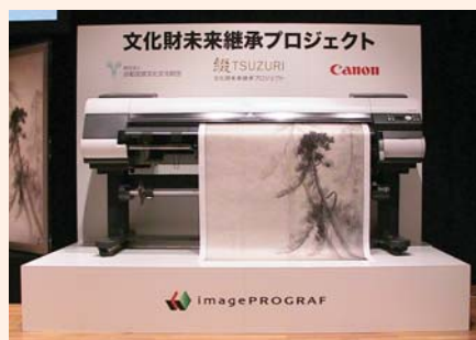
A large state-of-the-art digital printer reproduces an ink brush painting of pine trees drawn in the 16th-17th century on a folding screen, designated as a national treasure.
