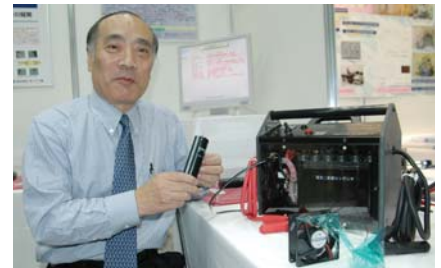
Prof. Morinobu Endo, the developer of technology to mass-produce carbon nanofiber, sits with a prototype engine starter that has replaced the conventional lead battery with a carbon nanofiber capacitor.
