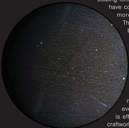
Microcracks detected by microscope x50
