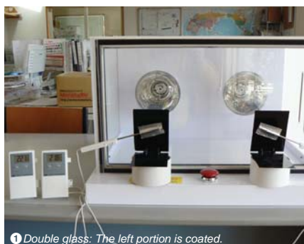
① Double glass: The left portion is coated.
