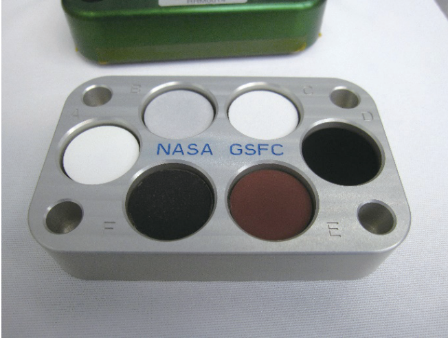
NASA tests carbon nanotube coating (slot "D" on sample tray) to make spacecraft instruments more sensitive without enlarging size.
