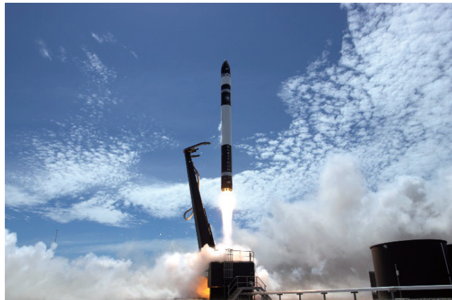
Rocket Lab's Electron rocket utilizes carbon fiber for the rocket's outer shell and 3D printing for the rocket's engines.
