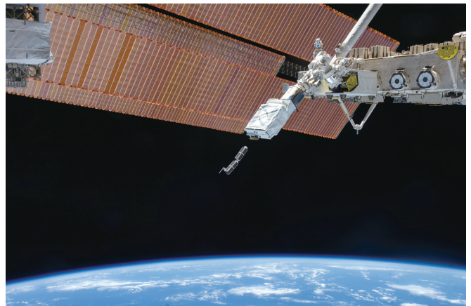
A pair of CubeSats deploy from the Small Satellite Orbital Deployer held by JAXA's Kibo laboratory robotic arm on the ISS.
