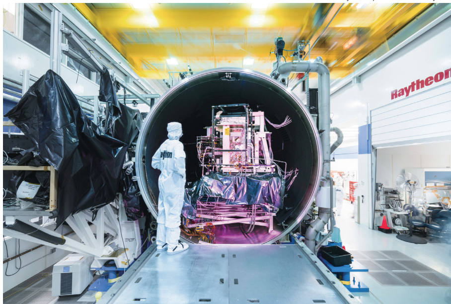
Raytheon Space Systems VIIRS instrument goes through rigorous testing to ensure it is ready for space. Here a Raytheon engineer inspects the JPSS-2 VIIRS instrument following testing in the thermal vacuum chamber.
