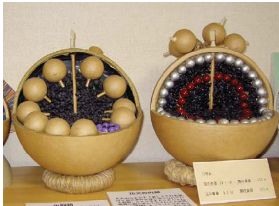
Sectional view of Japanese round shell fireworks. (left) Environmentally-friendly shells made of recycled paper. (right)
