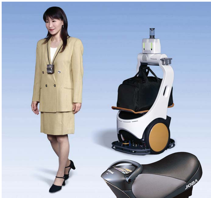
A porter robot (prototype) A typical tool-type robot that carries luggage and follows its possessor
