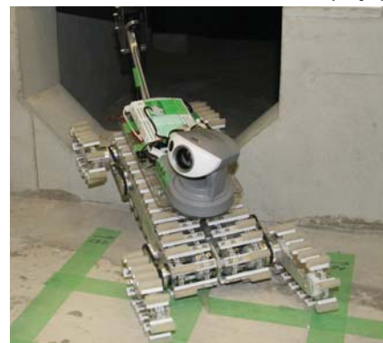
“Iris” is a downsized version of “Hibiscus” intended for home underfloor inspection.
