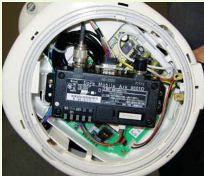
Mobile Ark, a wireless communication tool, is inside the i-POT
