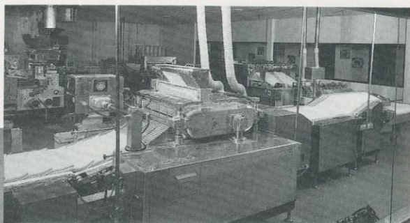
Part of the Rheon process of making dough for croissants, called the "MM Line"
