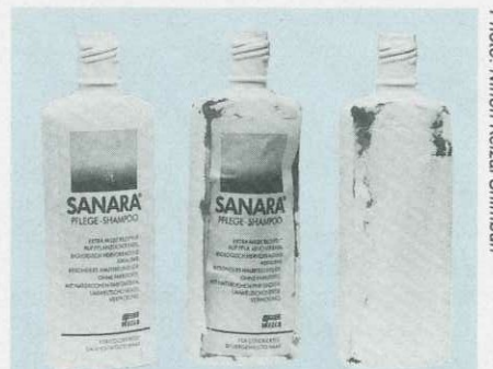
Shampoo bottles made of biodegradable plastic which is produced from the sugar content of agricultural products fermented by microorganisms. The bottles are degradable when placed in soil. The two bottles on the right are in the process of decomposing.
