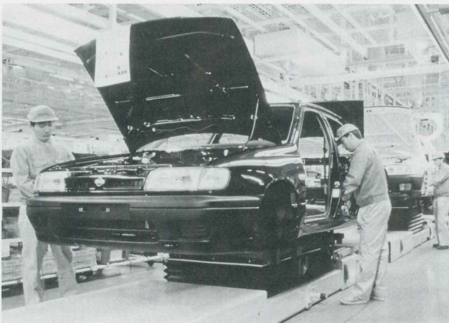
The challenges which face the auto industry in its drive to reorganize and rationalize: Nissan closed its Zama plant in favor of concentrating on the factory in Kyushu where motor-driven dollies are used on the assembly line.
