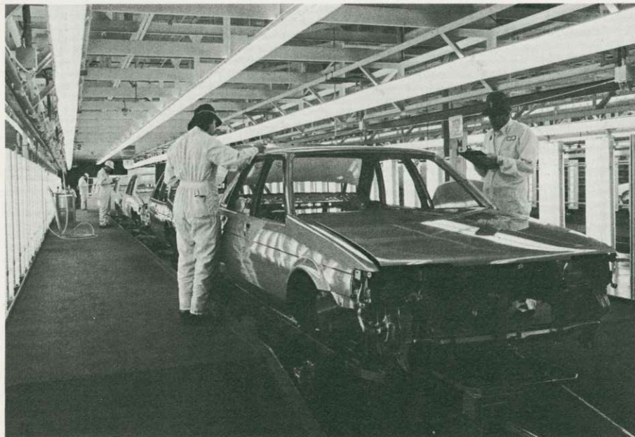
NUMMI's paint inspection area; defects are fixed immediately, right where the car is at.
