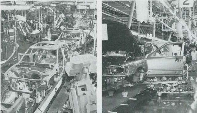
Intensive, large-scale assembly of the parts produced by the various group manufacturers is undertaken at domestic and foreign plants: body welding (left); assembly (right).
