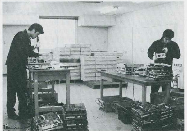
Preparing for the eco-production era: NEC's disassembly of personal computers
