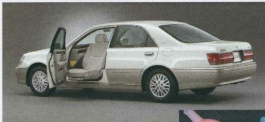
A vehicle with a rotary and movable front passenger seat (Toyota Motor Corporation)
