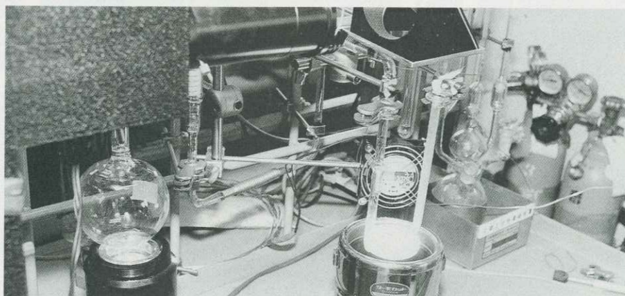
Photoreduction system of carbon dioxide that turns gases such as methane into fuel
