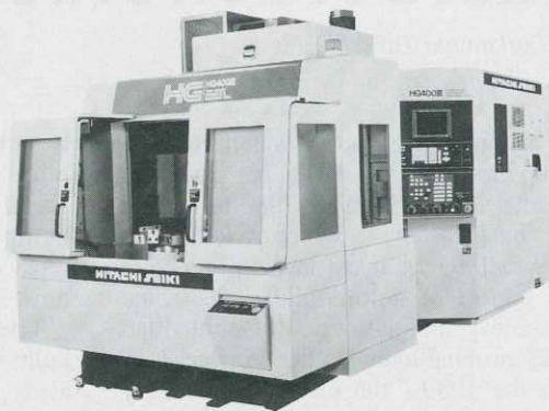
Man-made artisan: Skilled "hands" of machining center turn out many kinds of products in small quantities
