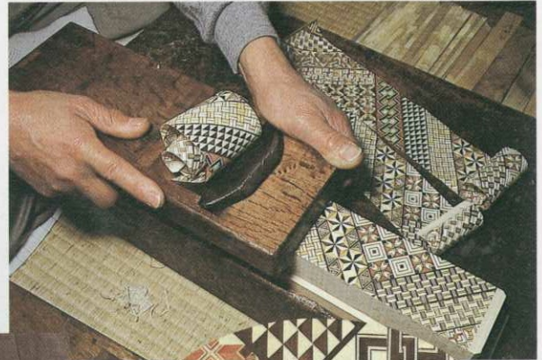
Top right: End-grain veneers curl from the plane
