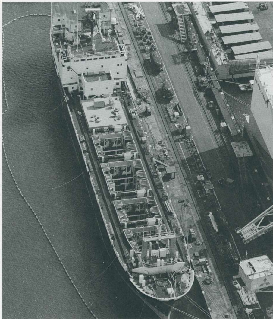
The Pacific Crane , berthed at a dockyard in Yokohama, is now being converted into a plutonium transport vessel, with state-of-the-art high-tech equipment and safety features including a reinforced hull.
