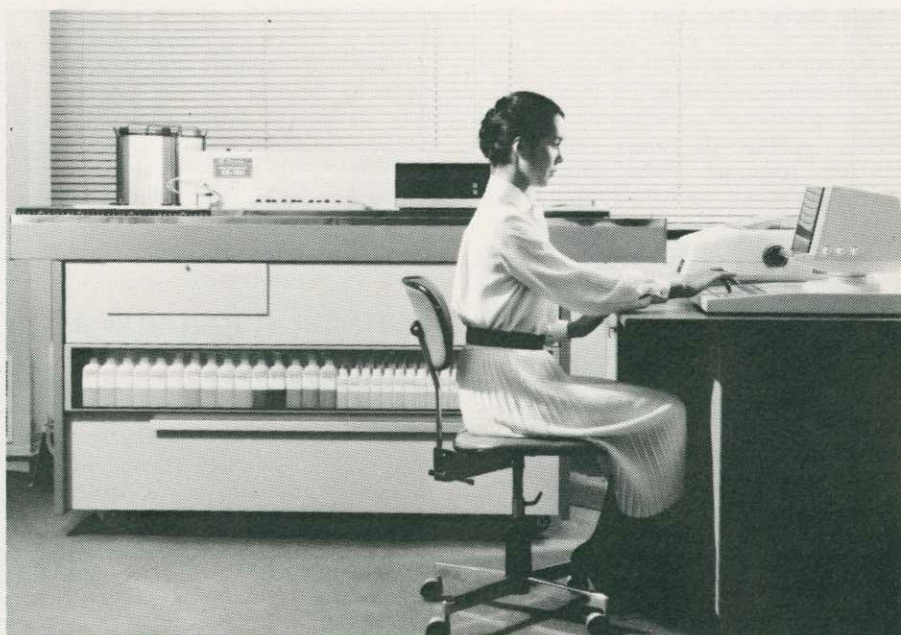
Photo 5: The world's most sophisticated testing device that can carry out 30 types of tests on 300 specimens per hour, or 9,000 tests per hour.
